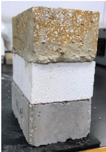
Fig.5. The 4-layer structure was used to validate the test method of effective elastic modulus.
